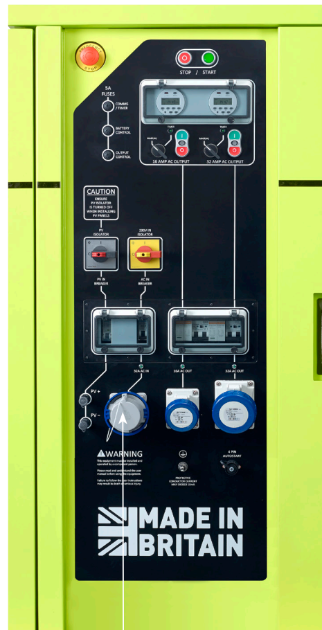
Connect 3 pin standard single phase (230V) cable to the 32A input socket and then to 32amp single phase output on generator
